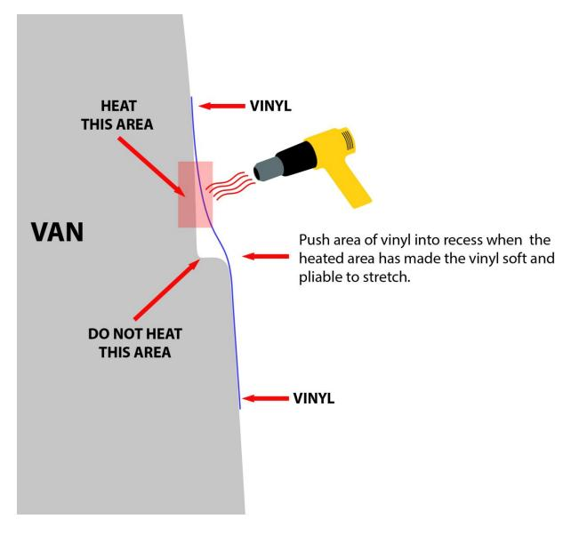
To apply vinyl to a recess, the material should be applied on top of the recess without stretching. The material should then be heated above the recess and the material stretched on the flat/straight section. The material should then be fed into the recess without any need to stretch/stress this area. After application the section should be post heated to "set" the vinyl.
