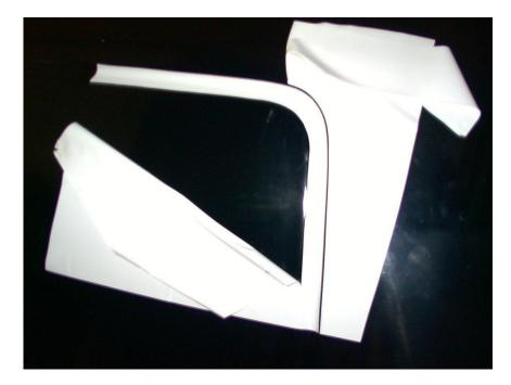
Apply VWS over the panel and recess. Cut a strip of the film (fillet) wide enough to fit into the recess and internal edges allowing material for trimming. Remove the excess material leaving the fillet. Working from the centre of the recess outwards in both directions, squeegee the vinyl into the base of the recess, around the internal radii and up to the outside edges of the recess. Remove the waste from the panels
